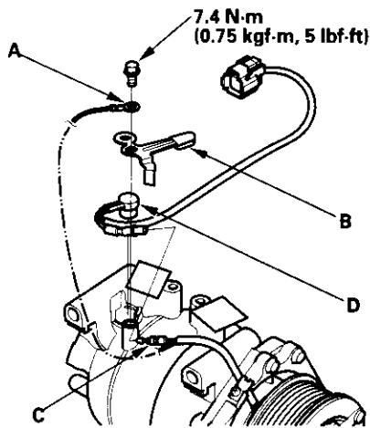
2. Replace the thermal protector (A) with a new one, and apply silicone sealant (B) to the bottom of the thermal protector.
